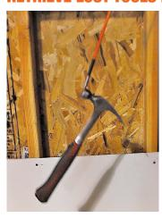
Magnetic Fish Rod Tip is strong enough to pick up a framing hammer lost in the wall.
